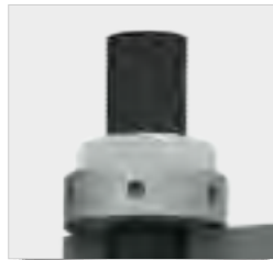
The nut rotating socket is assembled over the hexagon nut.
