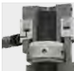
The pressure is released, the bolt is tensioned.
